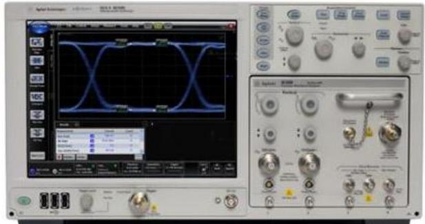
The image shows the Agilent 86100D Signal Analyzer with module 86108B. It features a color LCD screen displaying a graph with two overlapping curves. The device has a complex control panel with numerous buttons, knobs, and ports on the right side. |
