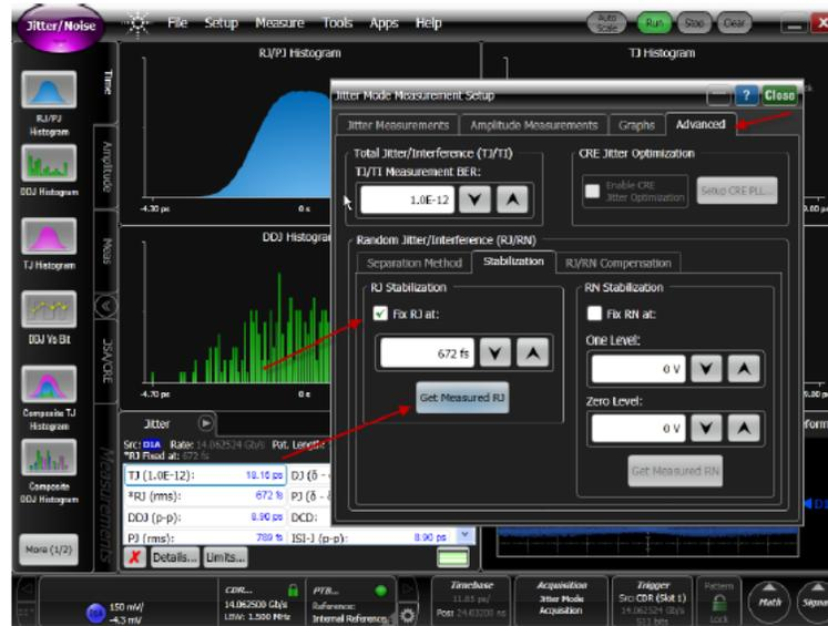
Figure 1. Locking the RJ value for long pattern measurements
