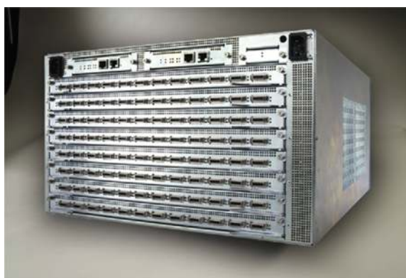
Figure 2. Cisco SFS 7008 Back Side, with Switch Ports and Redundant Power and Management
